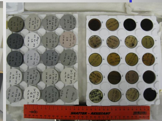
Pressed Pellets and Glass Beads for XRF
